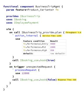
Figure 2: A sample component in the  $IET_S^3$  notation, supporting calls (regular component connections), triggers (performance analysis specific methods) and variant specific resource demands. The yellow boxes show attached analysis results.
